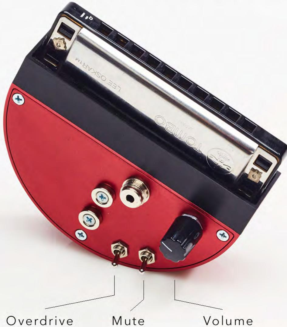
A Firebird model has a volume control, mute switch and an overdrive boost switch. The overdrive boost is adjustable via a small blue pot that is found on the pre-amp inside your Dyna-Mic. Turn this pot anti-clockwise for more overdrive.
